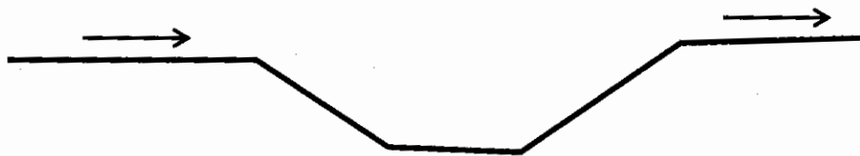
Figure Q4-1: Sewer system crossing a valley
