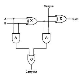
The above cirucit diagram shows a *full adder*. The gates marked X are exclusive or (XOR) gates; those marked A are AND gates; the gate marked O is an OR. Write out a truth table showing values of the *sum* and *carry out* for all the possible combinations of A, B and *carry in*. [8]
