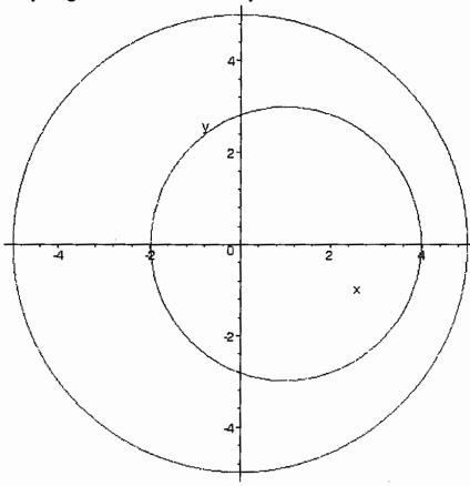
The outer hollow cable is having a radius of 5 and centred at the origin while the inner cable is having a radius of 3 and centred at x = 1 & y = 0.
