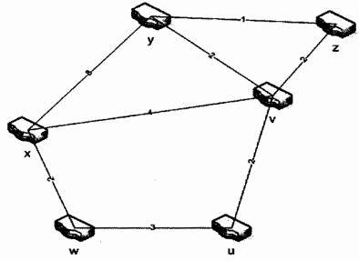
With the indicated link costs, use Dijkstra's shortest-path routing algorithm to compute the shortest path from node u to all network nodes. Hence create the routing table for node u.
