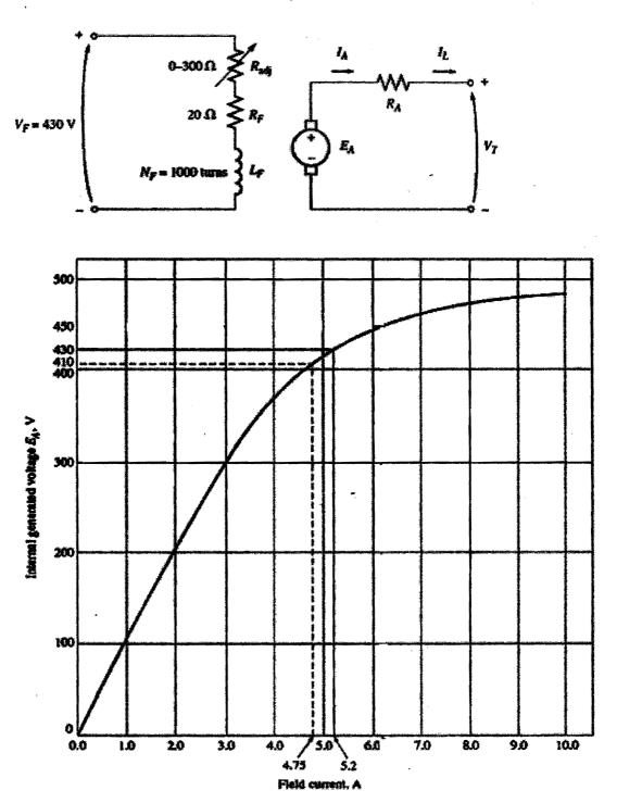
If  $R_{adj} = 63 \Omega$  and the prime mover speed=1200 rev/min,
