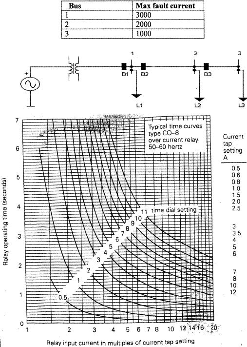
a) Calculate the tap setting for breaker B3.
