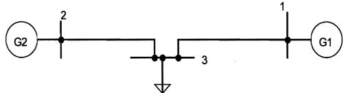
a) Find the admittance matrix of the system Ybus. Note: You don't need to derive the Ybus matrix. b) Solve for the first iteration of  $V_2$  using Gauss Seidel method.
