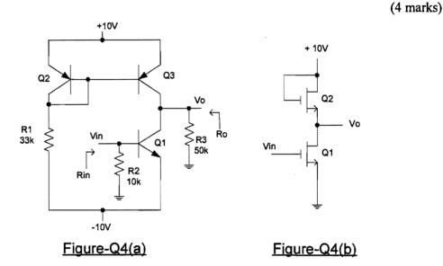
(b) A circuit of an enhancement type NMOS amplifier is shown in Figure-Q4(b). Some useful parameters of the devices used in the circuit, are shown below.
