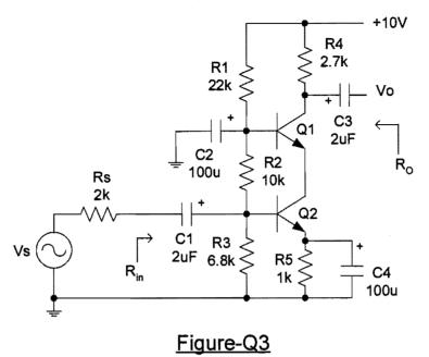
A circuit of a cascode BJT amplifier is shown in Figure-Q3.
