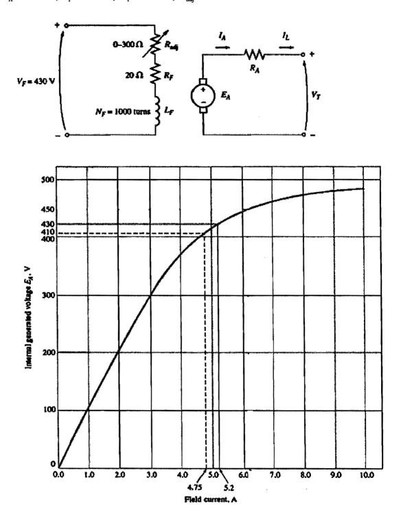
If  $R_{adj} = 63 \Omega$  and the prime mover speed=1400 rev/min,
