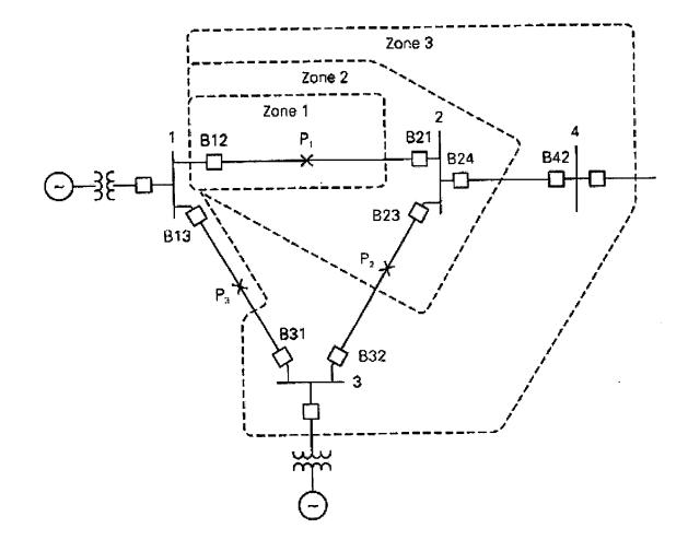
a) Determine the three impedance relay zones settings at breaker B12  $Z_{r1}$ ,  $Z_{r2}$ ,  $Z_{r3}$ , and time delay for the relay to trip in each zone.
