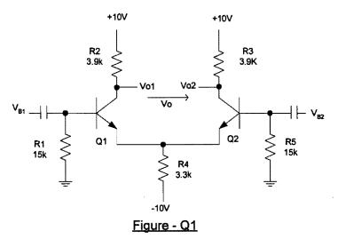
(a) Assuming that the transistors are of high gain type and matched, find the collector currents of the two transistors at no signal. Also find the voltages at the collectors and at the emitters.
