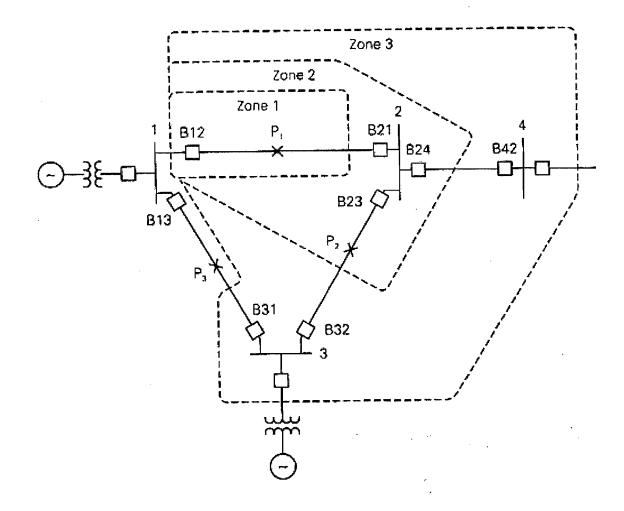
a) Determine the three impedance relay zones settings at breaker B12 ( $Z_{r_1}$ ,  $Z_{r_2}$ ,  $Z_{r_3}$ ) and the time delay for the relay to trip the circuit breaker in each zone.
