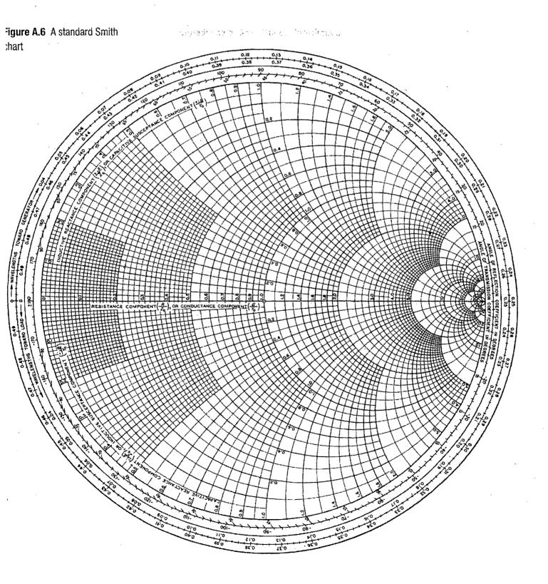
Q4: (20 pts) A lossless TV transmission line of 75  $\Omega$  feeds a dipole antenna of impedance 70+j40  $\Omega$ . (i)(5 pts). Find VSWR. To improve the VSWR design a  $\lambda/4$  transformer inserted in somewhere in the transmission from the load, (ii)(10 pts). Calculate the location from the load to put the  $\lambda/4$  transformer, (iii)(5 pts). the  $Z_o$  of the transformer.
