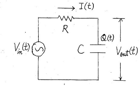
The circuit equation is  $V_{in}(t) = R \frac{dQ(t)}{dt} + \frac{Q(t)}{C}$  ..... (1) where  $I(t) = \frac{dQ(t)}{dt}$ . (i) Substituting  $V_{in}(t) \& Q(t)$  by  $V_0 e^{i\omega t} \& \hat{Q} e^{i\omega t}$  respectively into eq.(1) to solve for  $\hat{Q}$  in terms of  $V_0$ , R,  $C \& \omega$  and show that
