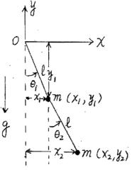
The kinetic and potential energies for the system in terms of  $x_1$ ,  $y_1$ ,  $x_2$  &  $y_2$  are  $T = \frac{1}{2}m(\dot{x}_1^2 + \dot{y}_1^2) + \frac{1}{2}m(\dot{x}_2^2 + \dot{y}_2^2)$  &  $U = mgy_1 + mgy_2$
