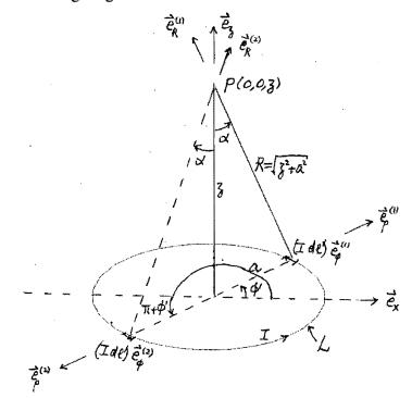
where  $\vec{e}_R^{(1)} \& \vec{e}_R^{(2)}$  are the unit vectors pointing from the small line segment current sources  $(I d l') \vec{e}_{\phi}^{(1)} \& (I d l') \vec{e}_{\phi}^{(2)}$  respectively to the field point P (0,0,z).
