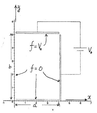
Its electric potential f(x, y) in Cartesian coordinates for the region between two conductors, i.e.,  $0 \le x \le a \& 0 \le y \le b$ , satisfies the following two dimensional Laplace equation :
