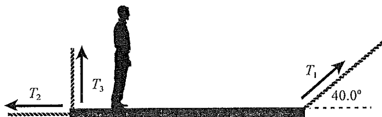
Figure 3. Person standing on a suspended plank.
